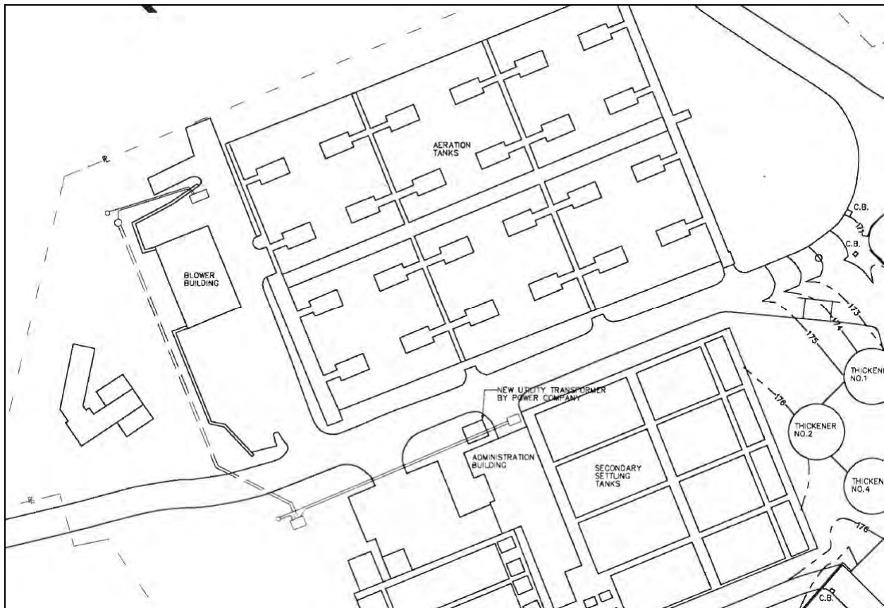
FIGURE 3-4 AERATION AND SECONDARY SETTLING TANKS
